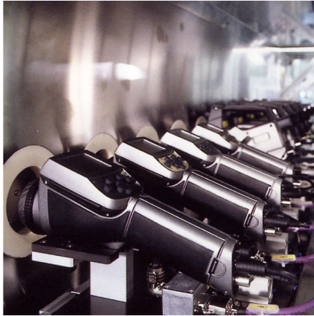
Figure 19.4 LEFT: Testing of infrared cameras in the climatic chamber; RIGHT: Robot used for camera testing and calibration
