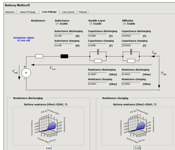
Graphical parameterization of the battery model in dSPACE ModelDesk.
