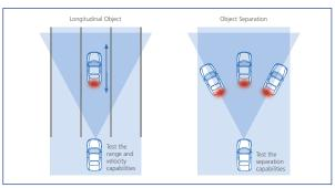
Performance and plausibility tests with radar sensors.
