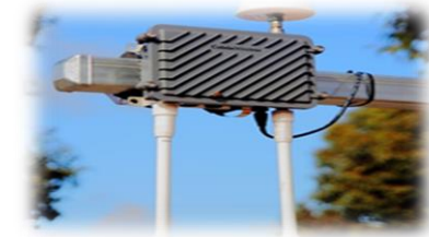
RSU(Road Side Unit)
